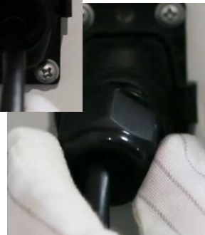
IP66 cover with rubber seal for RJ45 plugs
