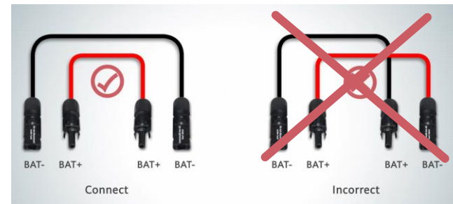
2x male for minus cable and 2x female for plus cable
